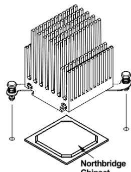
3. Align the push pins on the link assembly with the holes on the motherboard and fasten the bolts.
