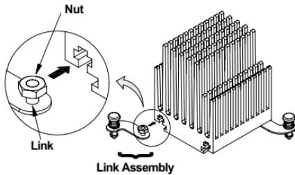
1. Insert the bolt into the bolt hole of the link and screw on the nut as shown in the diagram. Then, assemble the push pin and the spring onto the link. (The end of the spring having the smaller diameter goes with the head of the push pin.)
